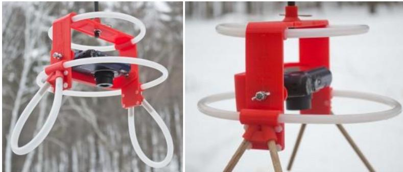
The traditional configuration is with four legs which protect the camera from dirt and wet grass during setup and against hard landings. There are two sizes of tubing — the thicker one is only for leg loops to replace the oak dowel legs (use short dowel pieces to attach loops to the brackets).
