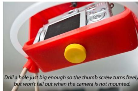
The thumb screw must turn freely in the hole before you try to thread it into the camera or you risk stripping the threads in the camera's tripod socket. But a tight fit prevents the thumb screw from falling out of the tray when the camera is not mounted. If the camera mounts too far from the lip, enlarge the hole toward the lip so the camera can be screwed on snug against the lip.
