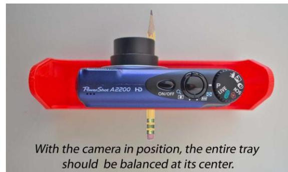
Balance the tray on a pencil as shown with camera back against a lip. Mark the location of the tripod socket on the tray (this requires a few steps of measuring and marking – see the [Redstone Rig Kit guide at kaptery.com/guides](http://kaptery.com/guides)).
