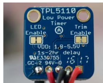
If you have a Log-a-Long Timer Kit see those instructions. To set the data logging interval on an Adafruit TPL5110 timer, use a small flat head screwdriver to gently turn the trimpot (looks like a Phillips head screw, below the flower and “TPL5110”). If turned all the way clockwise, the interval is short (less than a second). For testing, turn it all the way clockwise and then back a little. Don't force the trimpot, it's a bit fragile.
